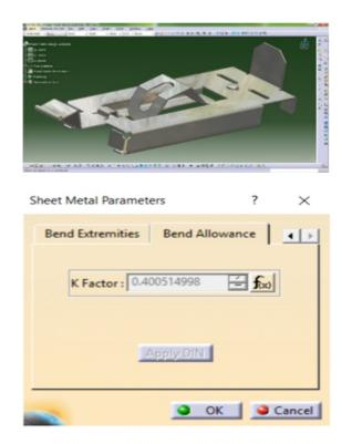
Bend allowance has a K factor, physically, the neutral fiber represents the limit between the material-compressed area inside the bend and the extended area outside the bend. This formula can be deactivated or modified by right-clicking in the K factor field and choosing an option from the contextual menu. It can be reactivated by clicking the Apply DIN button. Moreover, the limit values can also be modified.
