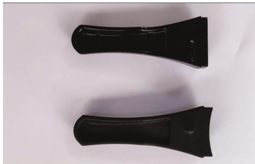
Prototype of Pressure cooker handle printed in Engineering Grade ASA Thermoplastic Material
