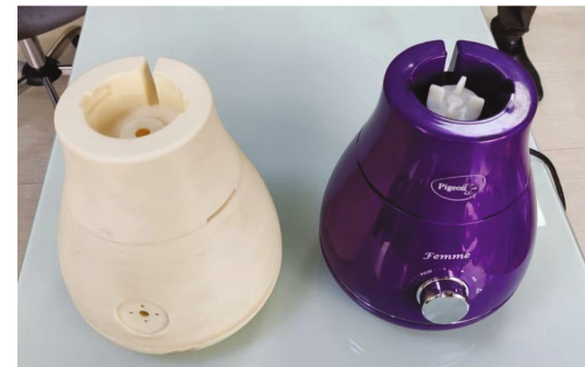
Prototype of Pigeon Mixer Assembly printed in Engineering Grade ASA Thermoplastic Material for design validation vs the Final model.
