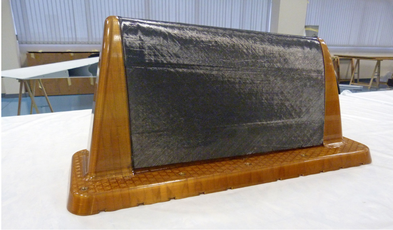
The preform tool offered perfect mechanical properties to resist high temperatures, enabling the team to reduce the carbon fiber heating stage from one hour to ten minutes.
