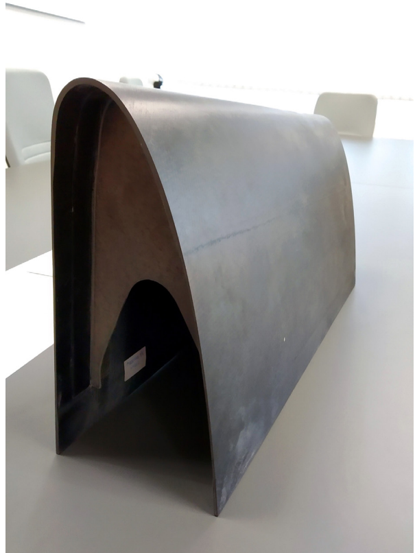
The final composite part of a curved aircraft wing, produced with FDM technology.
