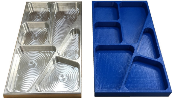
Figure 1: CNC (aluminum) on the left, 3D printed (plastic), right.
