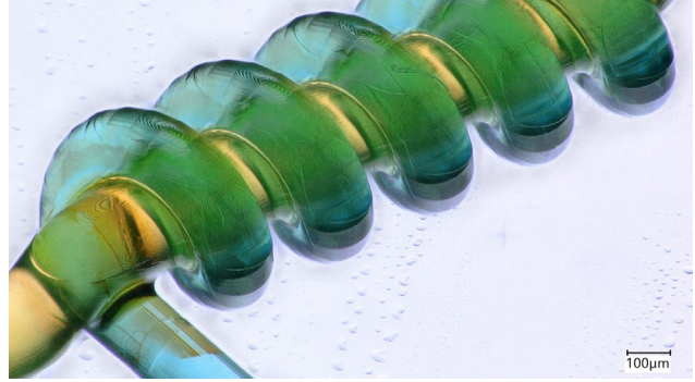
Effectively fabricate vasculature models with microscale printing.
