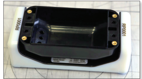
Figure 14: Heat-staked brass inserts in a plastic part held by a PolyJet fixture.
