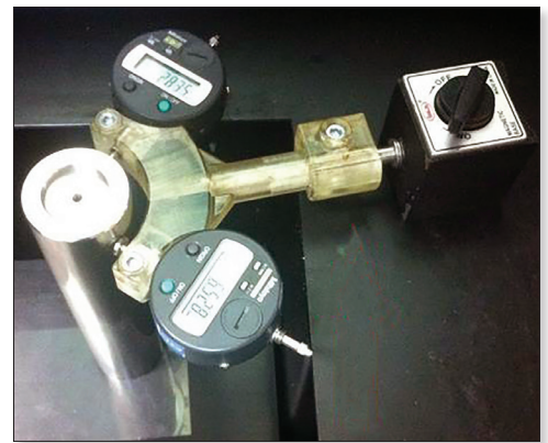
Figure 15: PolyJet 3D printed calibration fixture.
