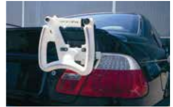
In the jigs and fixtures department at BMW AG, Regensburg, a Fortus system is used to manufacture assembly tools. This tool is used to affix the rear name badge.
