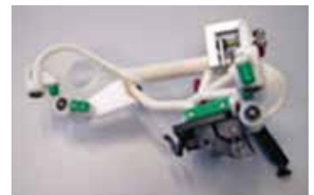
Produced with direct digital manufacturing, this tool is used to attach bumper supports.
