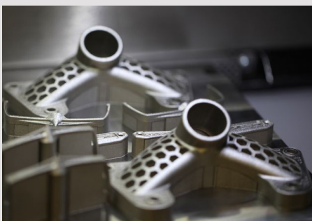
MPBD makes low-volume production feasible for complex metal parts. It can produce thin walls and other features that are difficult or cost-prohibitive to machine or cast.
