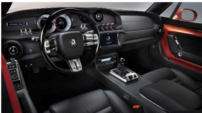
Many of these chrome interior details were created with laser sintering technology. Parts were electroplated to achieve a shiny metallic finish.
