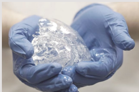
SL has empowered doctors at the Texas Cardiac Arrhythmia Institute to create accurate models of their patients' hearts before performing surgery.
